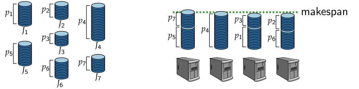
**Output.** Distribution of jobs to machines such that the time when all jobs have been processed is minimal. This is called the **makespan** of the distribution.
